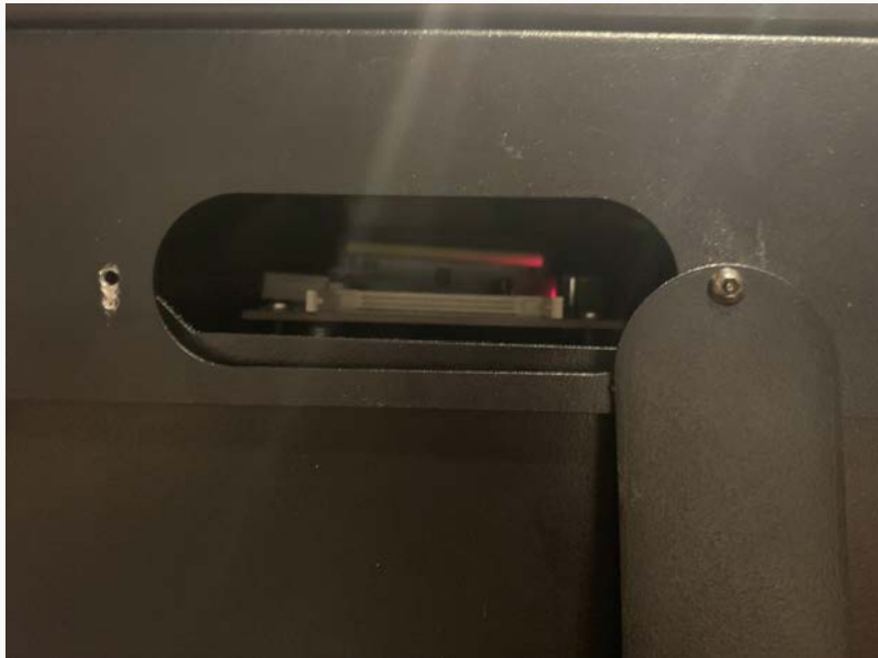
Picture: Small unmarked lid on the side of the machine for accessing CF card slot inside of the machine. So-called “secure screw” tips can be commonly purchased from any electronic store.
