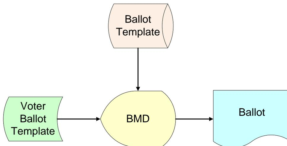
The ballot definition templates are files that are preloaded into each BMD by county elections personnel. The voter ballot template is typically a voter access card or bar coded paper with a ballot template ID that tells the election management system the voter is authorized to cast one vote. The bar coded paper serves the same purpose for many BMDs that the voter access cards server for DREs
